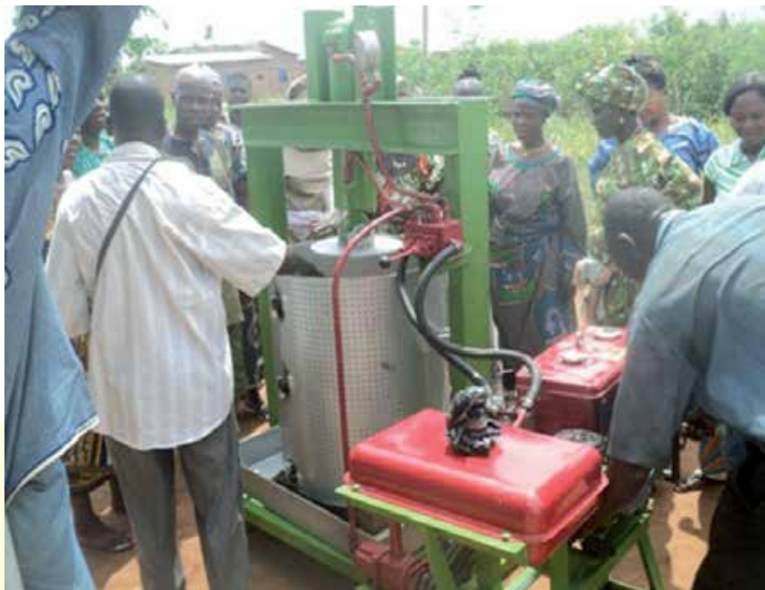
Women group being trained in Benin to use efficient cassava dough compressor
